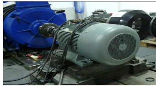
Fig. 1. Prototype of a three-phase induction motor during testing
